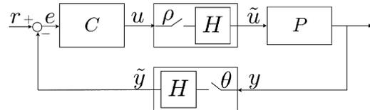
Fig. 1. Setup;  $P$ -plant,  $C$ -controller,  $\rho_t \in \{0, 1\}$ , and  $\theta_t \in \{0, 1\}$  determine if data losses occur at time  $t \in \mathbb{Z}$ ;  $H$  represents the hold scheme (3), (4), by which the most recently received data is hold constant in case of a data loss.
